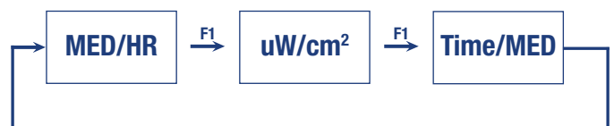
Figure 6 Pressing The F1 Function Key Converts The Measurement Result Into One Of The Available Unit Systems. UVB Detector Display Units Shown
